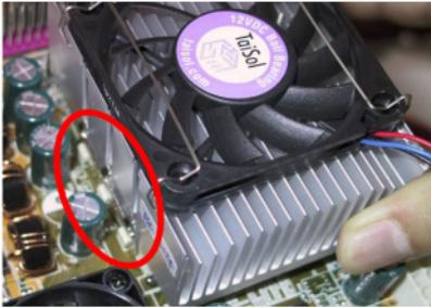
Insert the heatsink left side fix plate into the processor socket left side fix hooks. Make sure the fit is very tight. Check the photo on the left.
