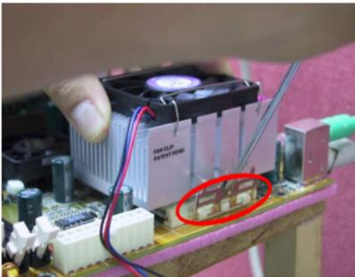
Check the photo on the left. You have finished the heatsink installation. Now hold the whole heatsink and slightly shake it, make sure the bottom right side of the heatsink does not contact the right side of the Socket (see bottom picture). Otherwise, the processor die does not have proper contact with the heatsink. This situation
