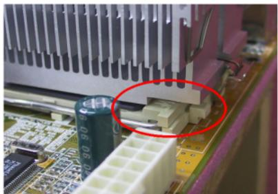
The left photo shows the bottom right side of the heatsink in contact with the right side of the Socket. In this situation, the processor die does not properly contact the heatsink. If you start the computer at this moment, it will immediately cause processor damage. Always check this location when you finish the heatsink installation.
